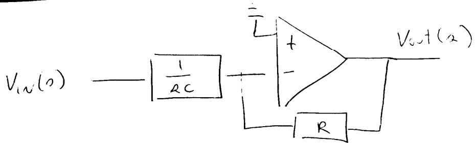
$$\frac{0 - V_{in}(s)}{1/RC} + \frac{0 - V_{out}(s)}{R} = 0$$
