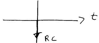
c) Output(s) =  $-R\omega C \cdot \frac{s}{s^2 + (10\pi)^2} = -RC \frac{\omega^2}{\omega^2 + (10\pi)^2}$
