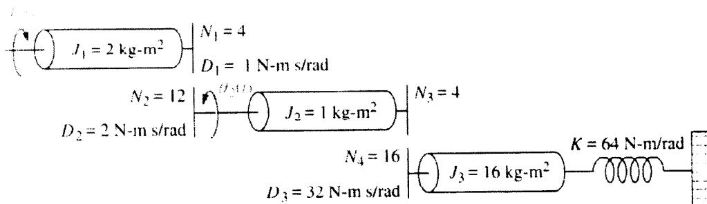
32. Find the transfer function,  $G(s) = \theta_2(s)/T(s)$ , for the rotational mechanical system shown in Figure P2.21.
