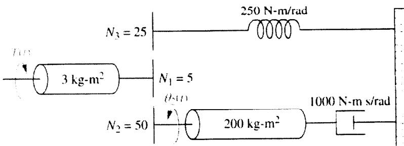
33. Find the transfer function,  $G(s) = \theta_4(s)/T(s)$ , for the rotational system shown in Figure P2.22.
