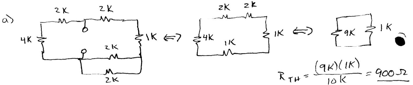
b)  $R_L = R_{TH}$  for MPT  $R_L = 900\Omega$
