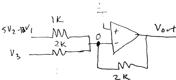
$$\frac{0 - (5V_2 - 12V_1)}{1000} + \frac{0 - V_3}{2000} + \frac{0 - V_{out}}{2000} = 0$$
