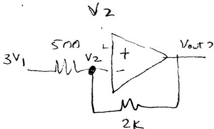
$$\frac{V_2 - 3V_1}{500} + \frac{V_2 - V_{out2}}{2000} = 0$$
