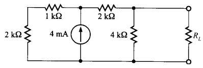
4.57 Find Rl for maximum power transfer and find the maximum power transferred.
