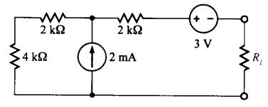
4.58 Find Rl for maximum power transfer and the maximum power that can be transferred in the following circuit.
