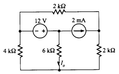
4.55 Find Rl for maximum power transfer and find the maximum power transferred to this load.
