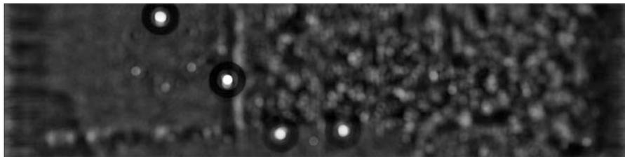
**Fig. 9** The test statistic computed on the input SAR image without masking detections
