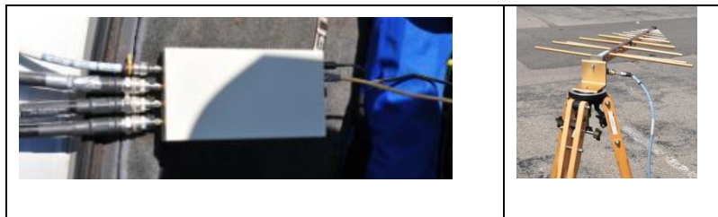
Figure 1. Experimental Radar. Left: Akela radar unit. Right: Antenna.
