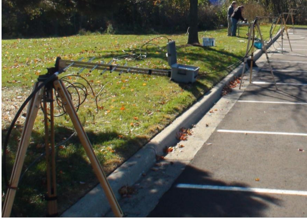
Figure 2. The Four antenna configuration used in this experiment.
