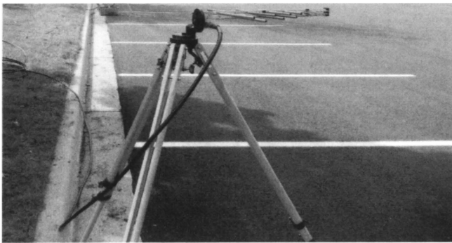
Figure 3. A Yagi log-periodic antenna, as deployed.
