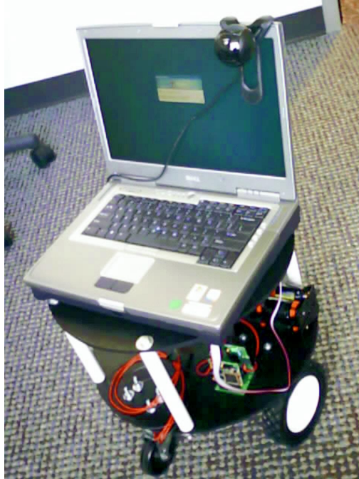
Figure 3. The Inverted UAV experiment described in this paper uses a wheeled ground robot that carries a standard laptop. The laptop executes the the sensor management algorithm described earlier and produces commands which dictate the movement of the robot. The low-level robot motion is controlled via a 16-bit CPU system which communicates with both the motor controller board and the laptop.
