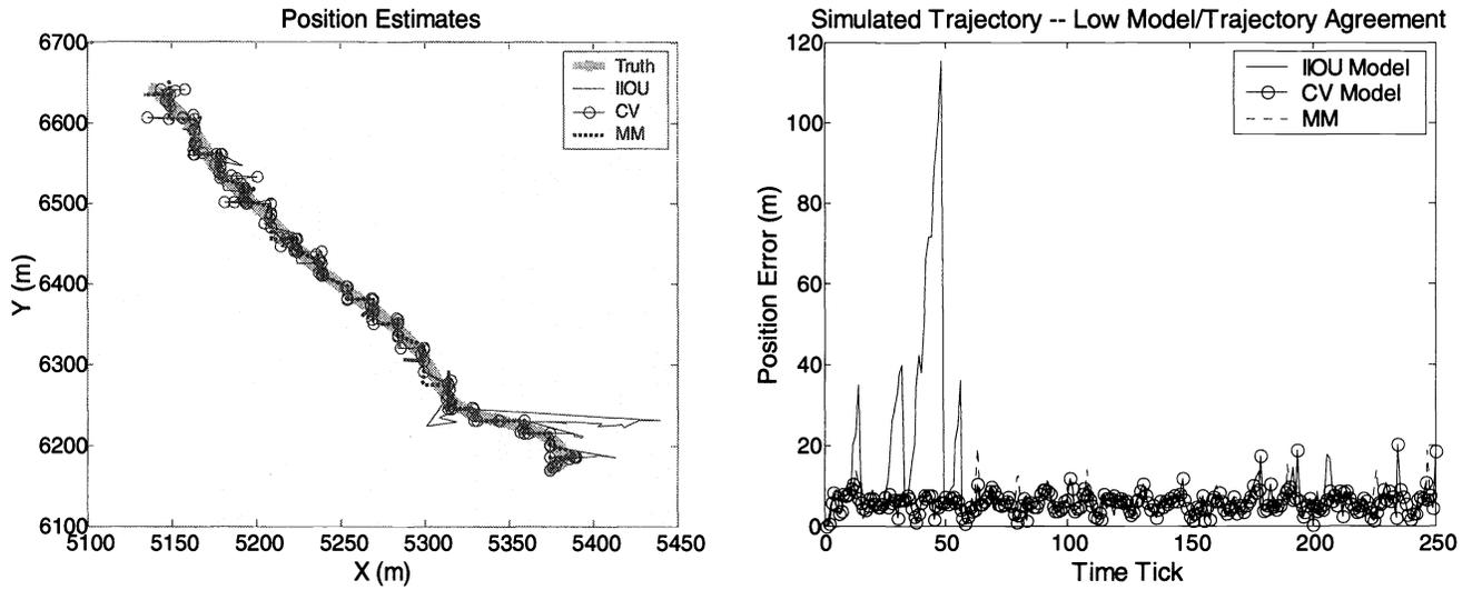
Figure 5. (L) The target trajectory and the different trackers position estimates. (R) The position RMSE for each time step.
