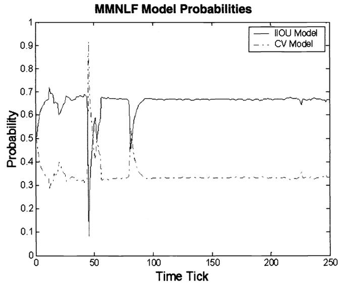
Figure 6. The model probabilities show that the filter mostly acts in the IIOU mode until the targets behavior warrants a switch to the CV mode at around  $t=40$ .
