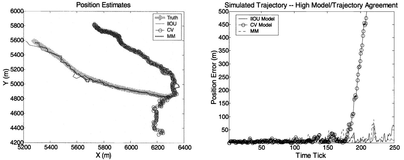
Figure 2. (L) The target trajectory and the different trackers position estimates. Both the IIOU and MM trackers hold the target, while the CV model loses it. (R) The position RMSE for each time step.
