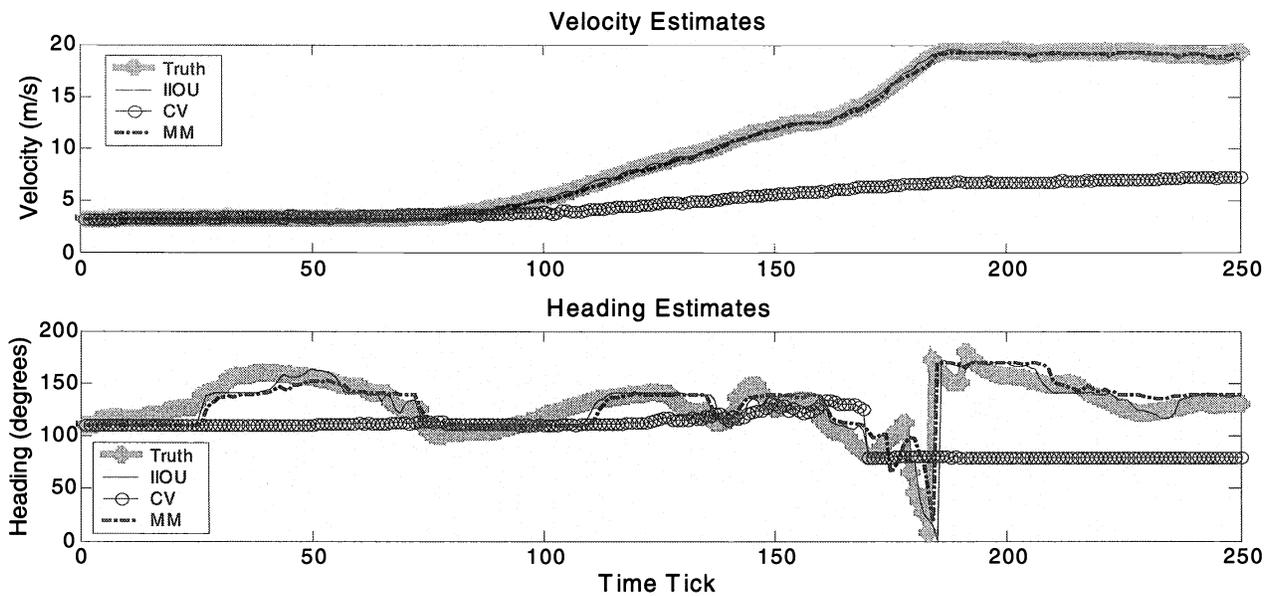
Figure 3. (T) The speed estimates of the three trackers show that the CV model is unable to hold on to the target as it speeds up. (B) The heading estimates show that the complicated maneuver at  $t=180$  causes the CV to lose track.
