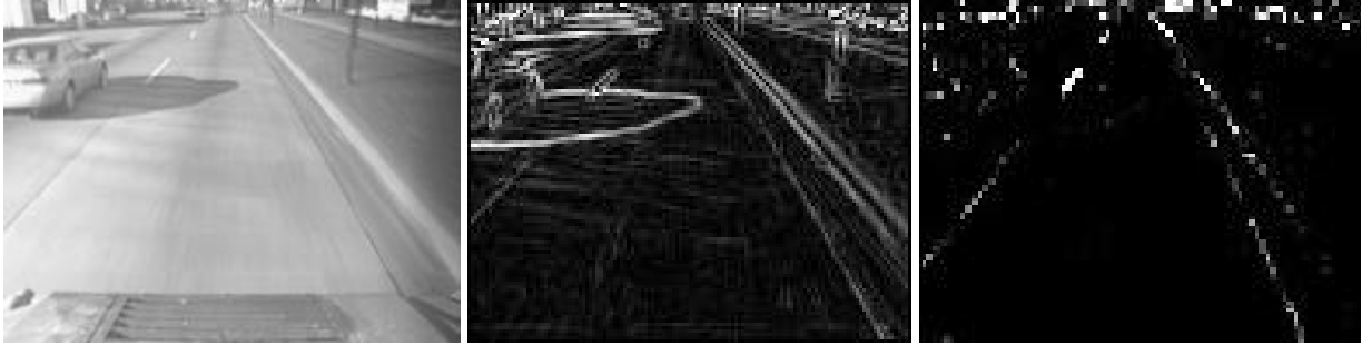
Figure 9. Left: A typical road image. Middle: The image’s gradient field. Right: The image’s new feature vector field.
