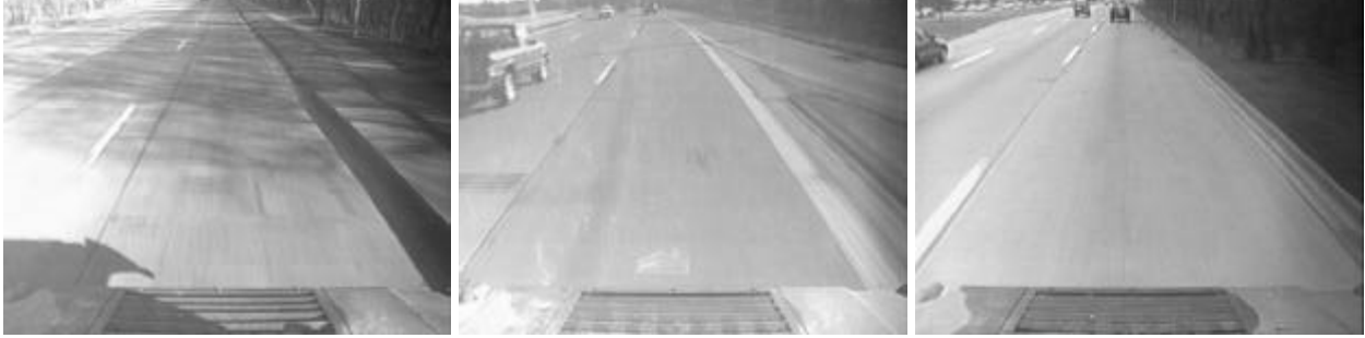
Figure 4. Examples of several roadway scenes to illustrate the fact that lane and pavement edges are oriented diagonally in the image plane
